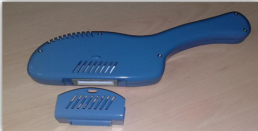
The finishes on the pieces are almost always manual post-process operations that affect the cost of the prototype. Of course if you need to have a particular aesthetic, you can not do without these operations; we can execute many finishes including varnishing, screen printing, vacuum metallization, anodizing polishing.
